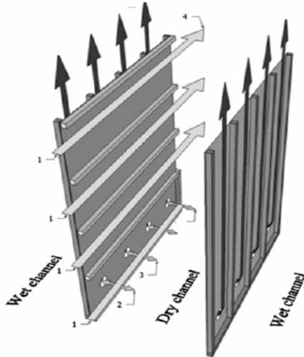
Fig 2: Wet and Dry Channels of M-Cycle Cross Flow Heat Exchanger
