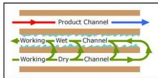
Fig 4: Working of M-cycle
