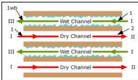
Fig 3: Cross section showing indirect evaporative cooling
