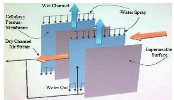
Fig 5: Cellulose porous stack heat exchanger configuration of a DPEC
