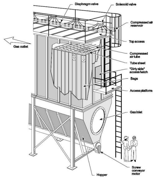
Figure: 1 Typical pulse jet fabric filter
