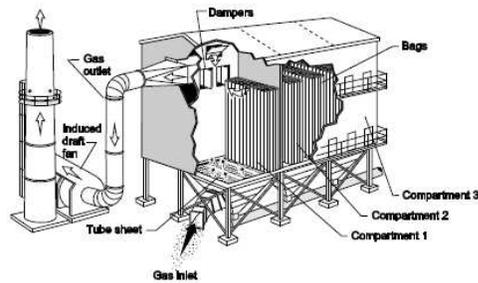
Figure 4: Reverse pulse jet fabric filter
