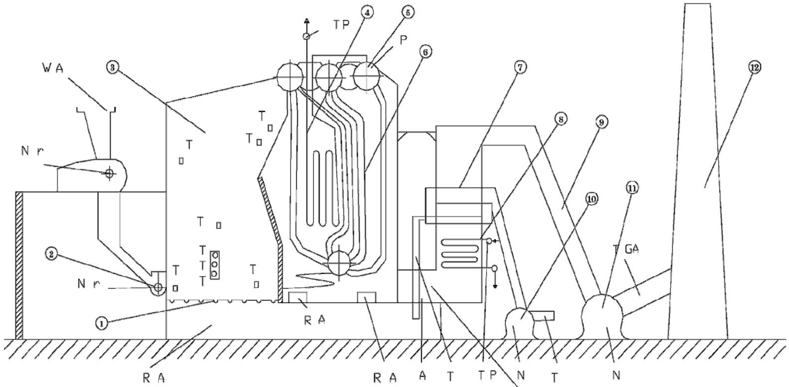
Bagasse fed to these boilers enters the furnace through five fuel chutes and is spread mechanically. The major part of the bagasse characterized by small and light pieces, burns in suspension. Simultaneously, large pieces of fuel are spread in a thin even bed on a stationary grate.
